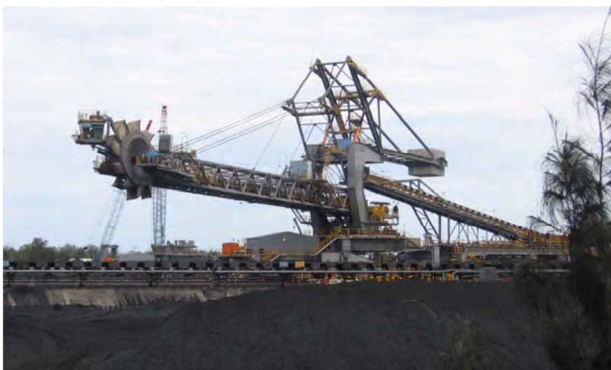
Figure 5: “C” frame stacker reclaimer
