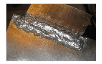
Welding defects can greatly affect weld performance and longevity, early detection and correction is important to ensure that welds can carry out their designed purpose.
