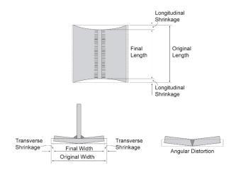
Common types of distortion include shrinkage, angular distortion and bowing. Causes of distortion include the heat input, the degree of restraint applied and inherent stresses in the parent metal.
