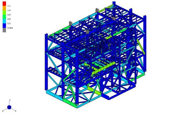
**Figure 10: Member Capacity Utilisation Ratios for a Module**
