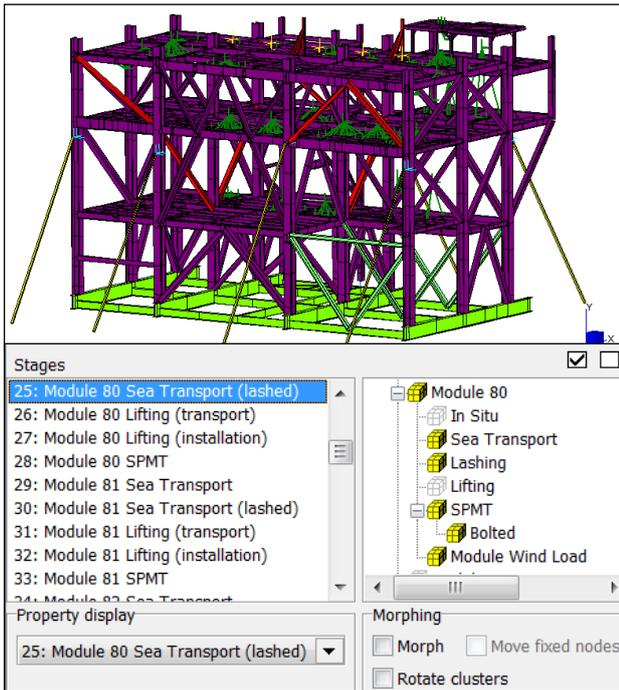
**Figure 11: Analysis Stage –Sea Transport of a Module**
