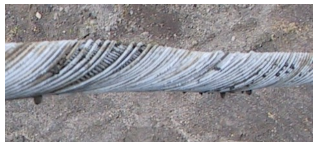
Figure 9 – Wire Rope Defect: Bird Caging
