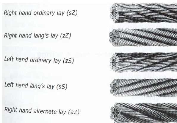
Figure 7 – Ordinary and Lang's Lay
