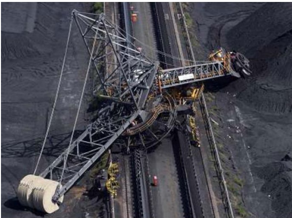
Figure 8: Machine Failure due to Fatigue
