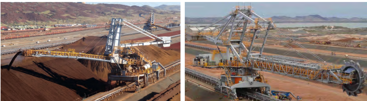
Stacker (Left), Reclaimer (Right)
