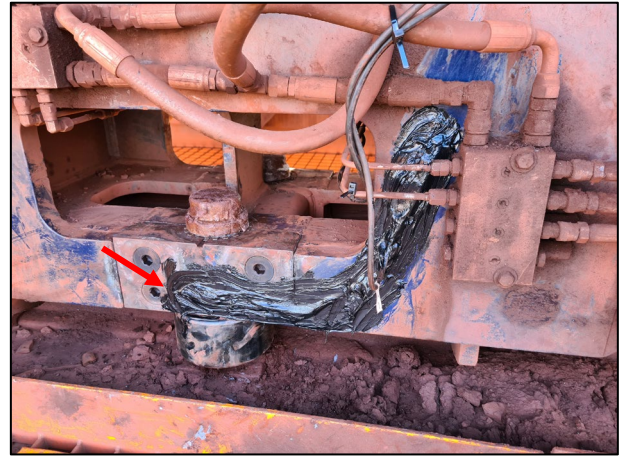
Figure 5 – Strain gauges were installed on the bogie structure, above the cam follower. Wiring was coated to protect the installation from physical damage.
