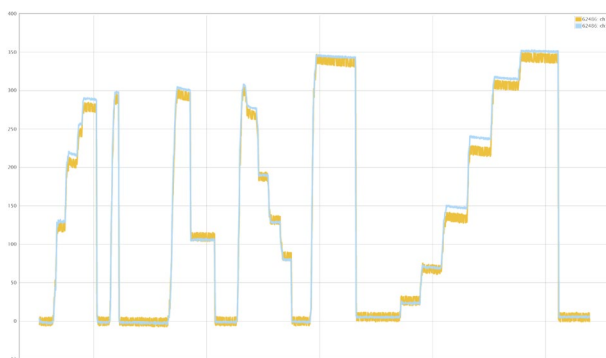
Figure 4 – The system was calibrated in the workshop by measuring strains in the bogie for known applied loads.
