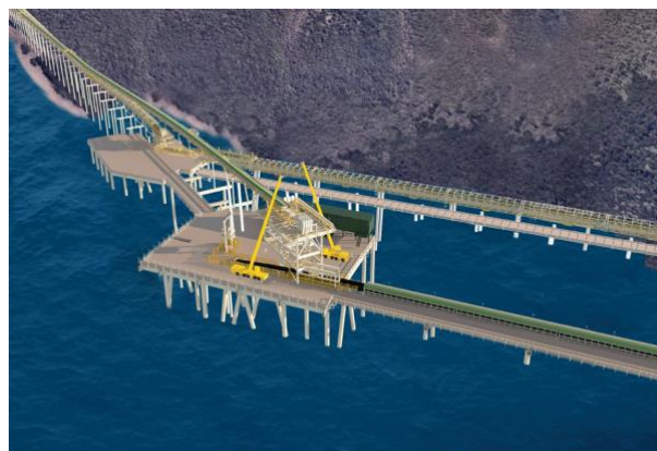
Figure 17 Crane Lift Configuration on Transfer Deck
