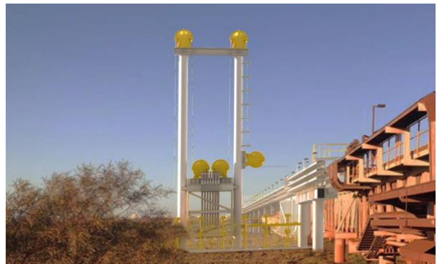
Figure 14 CVR 261 Gravity Take-up
